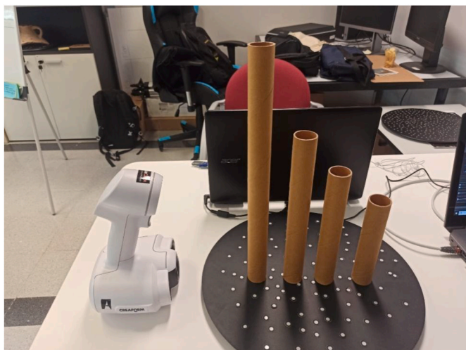
Fig. 2. Picture of some of the reference pieces used to characterize the volume uncertainty.
