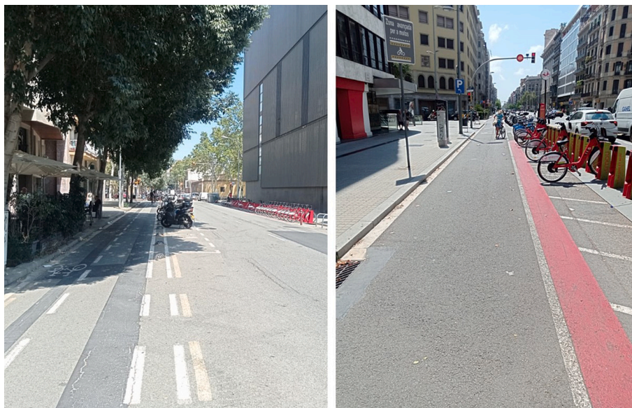
Image 8. To the left, example of docked station disconnected from the cycling network. To the right, example of docked station connected to the cycling network (source: author’s own).
