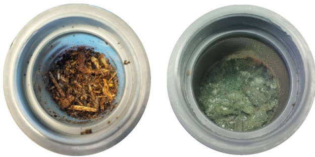
Fig. 1 SSF with T. viride on 0.5 L bioreactors
