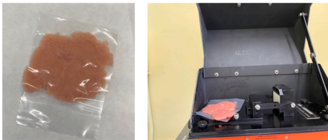
Fig. 2. Spectral acquisition of ground samples. Scanning setup showing the ground sample covered with a plastic film during near-infrared (NIR) analysis.
