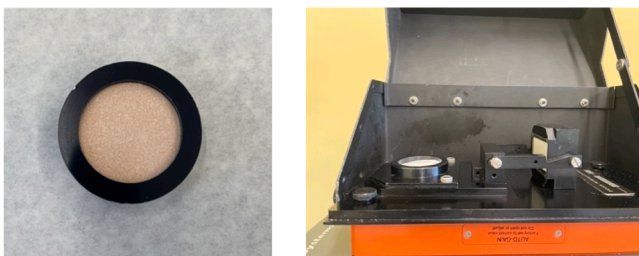
Fig. 3. Spectral acquisition of freeze-dried sample. Scanning setup showing the freeze-dried sample using a ring cup during near-infrared (NIR) analysis.
