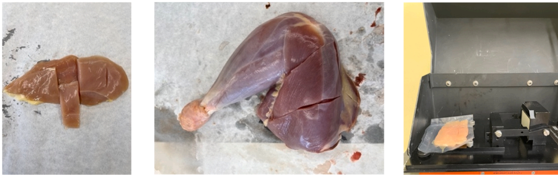
Fig. 1. Preparation and spectral acquisition of fresh meat samples. Standardized piece ( 8 \times 5 \times 1 cm) cut from the breast (left) and thigh (middle). Right: scanning setup showing the sample covered with a plastic film during near-infrared (NIR) analysis.
