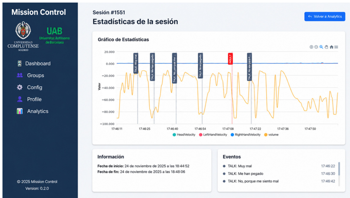
Figure 3. Exportable analytics graph of a session in the Mission Control dashboard. The session statistics dashboard shows movement-derived variables and behavioural events. Non-English interface labels appearing in the dashboard correspond to standard interface terms: “Estadísticas de la sesión” = session statistics; “Gráfico de Estadísticas” = statistics graph; “Información” = information; “Eventos” = events; “Fecha de inicio” = start date; “Fecha de fin” = end date; “Volver a Analytics” = back to analytics. Speech-related events (TALK) are marked by vertical annotations. The corresponding English translations are: TALK (17:46:22): ‘I feel very bad.’ TALK (17:46:30): ‘They hit me.’ TALK (17:46:42): ‘No, because I feel unwell.’ TALK (17:46:55): ‘I hit them.’ INSULT (17:47:10). TALK (17:47:20): ‘It wasn’t for you, teacher, sorry.’
