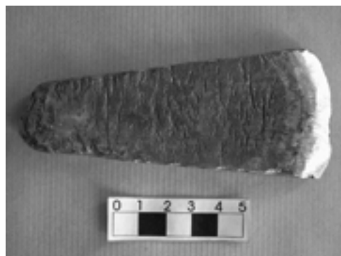
Fig. 4. Bronze flat axe after forging (5% tin).
