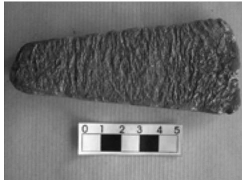
Fig. 2. Untreated bronze flat axe (5% tin).
