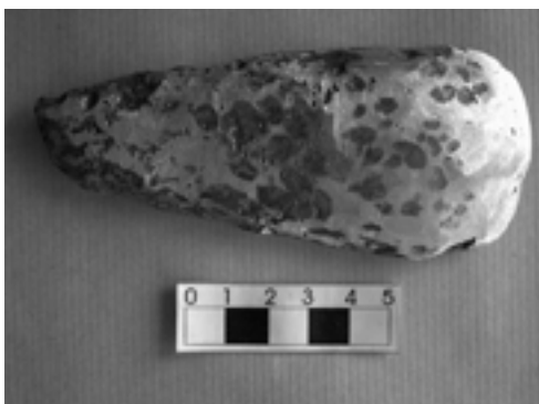
Fig. 3. Copper flat axe after forging.
