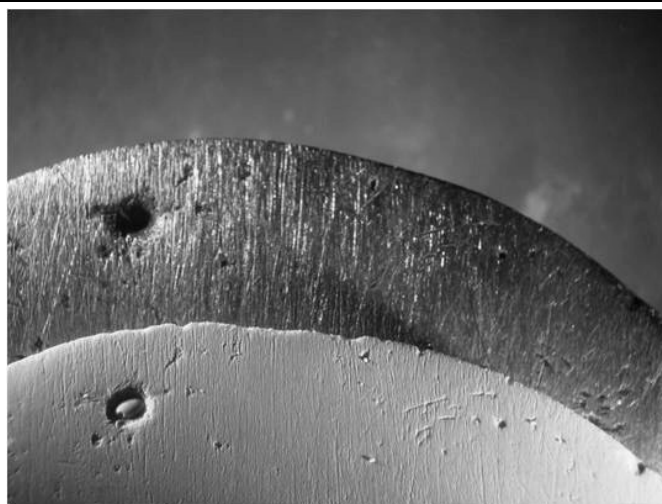
Fig. 18. Technological notches on silicon rubber mould of an axe before use. Technological notches modified after use, bronze axe (17% tin) (10x)
