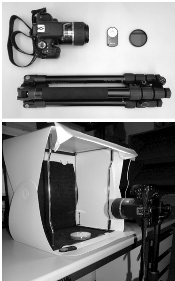
FIGURE 2. Photographic equipment employed to obtain the pictures of the Arvicola humeri. The camera with the macro lens, the polarising filter, the tripod, and the remote trigger separately (top) and mounted in front of the humerus fixed to the turntable inside the lightbox (bottom).
