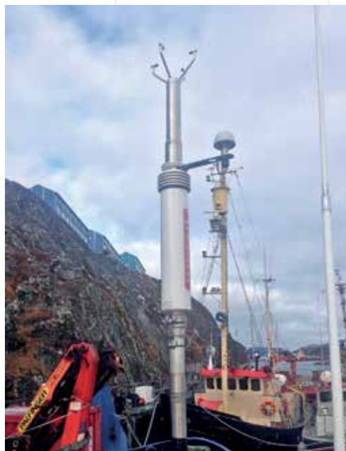
Figure 1. Left panel: the weather station mounted on the vessel Marie Martek. Right panel: Data display in the passenger cabin. Photos: Jakob Abermann.
