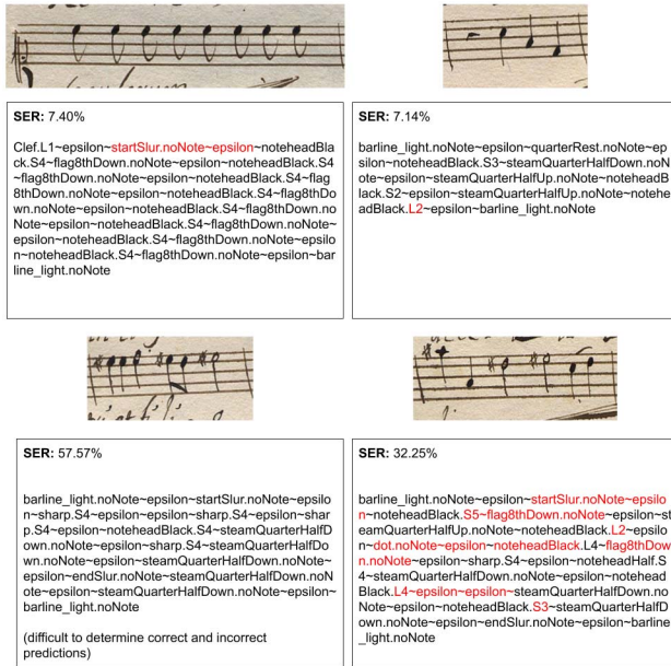
Fig. 7. Qualitative results. Mistakes shown in red color. From left to right and from up to down. First image: a slur is predicted instead of lyrics. Second image: the pitch of one notehead is confused. Third and fourth images: multiple mistakes because lyrics are too close to music symbols.
