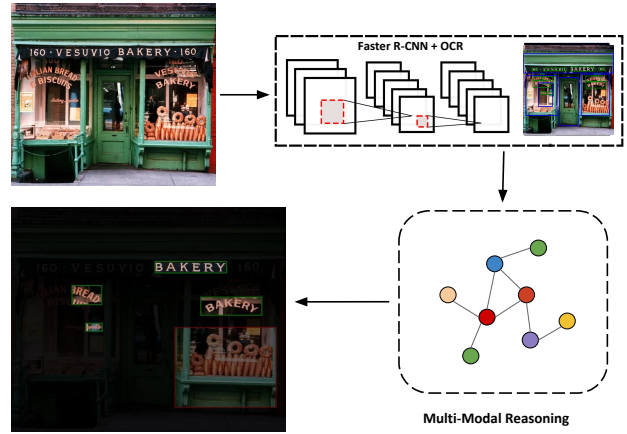
Figure 1. The proposed model employs a Graph-based Multi-Modal Reasoning (MMR) module to enrich location-based visual and textual features in a combined semantic representation. The network learns at the output of the MMR to map strong complementary regions of visual (red) and text (green) instances to obtain discriminative features to perform fine-grained image classification and retrieval.
