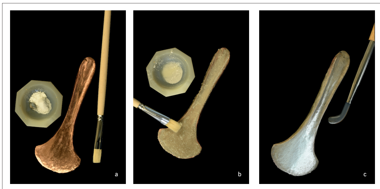
Fig. 23a–c Results of silver coating experiments. a silver chloride; b sodium chloride; c cream of tartar.
