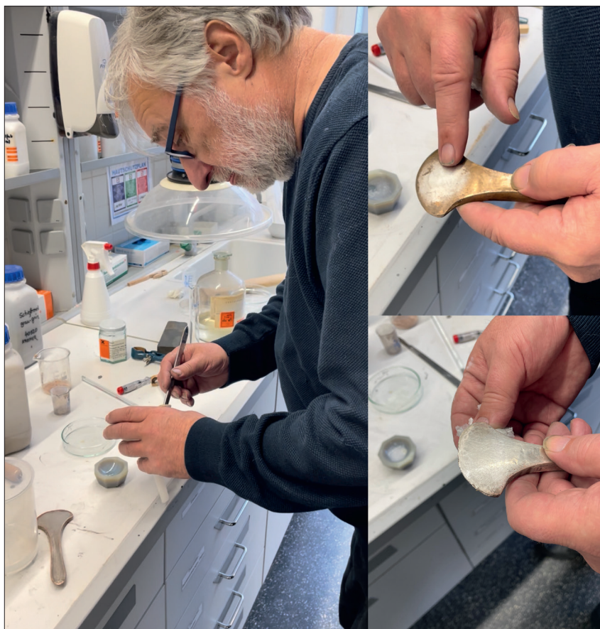
Fig. 22 Experiments of silver coating with silver chloride, sodium chloride, and cream of tartar.
