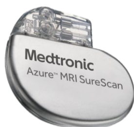
Figure 4 Example of a pacemaker currently on the market.
