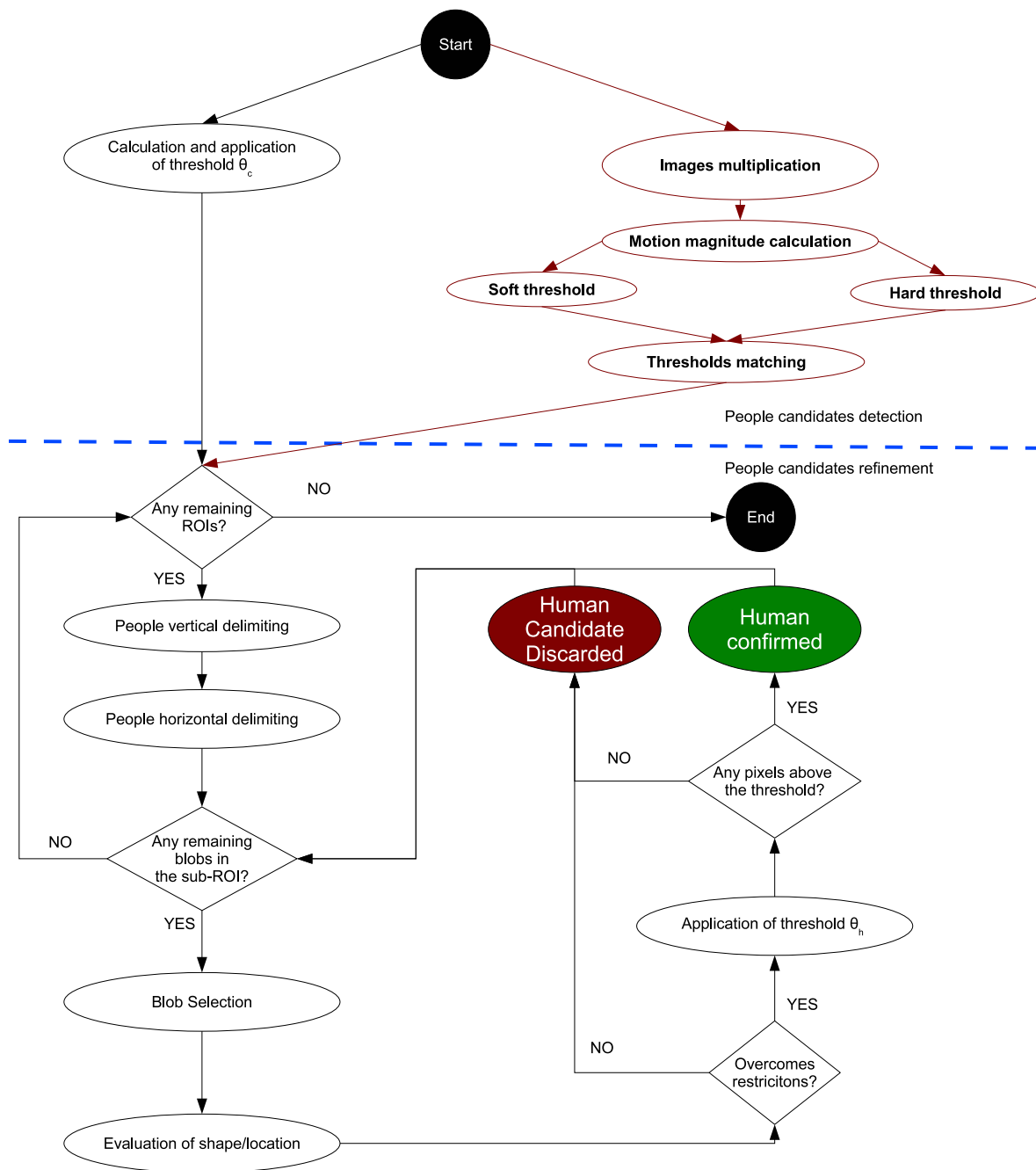
Figura 4.15: Algorithm of human detection in the infrared spectrum based on optical flow calculation.
