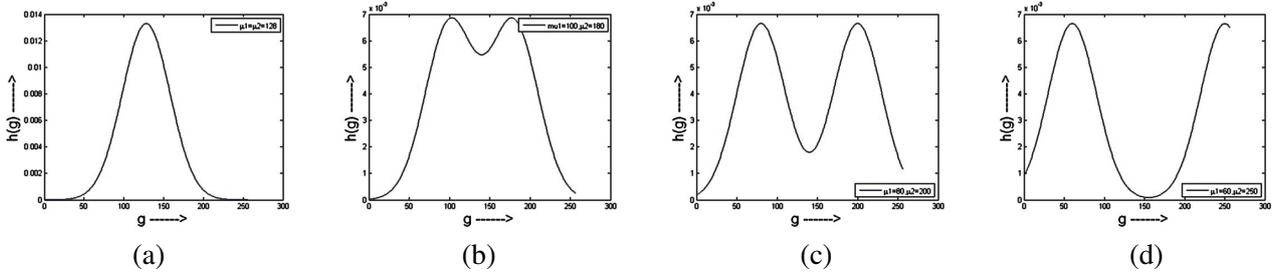
Figure 1: Simulated two class Gaussian Mixture PDF using (2)  $w_1 = w_2 = 0.5$ , and  $\sigma_1 = \sigma_2 = 30$ , with four different combination of  $\mu_1$  and  $\mu_2$ : (a)  $\mu_1 = \mu_2 = 128$ , (b)  $\mu_1 = 100$  and  $\mu_2 = 180$ , (c)  $\mu_1 = 80$  and  $\mu_2 = 200$ , (d)  $\mu_1 = 60$  and  $\mu_2 = 250$
