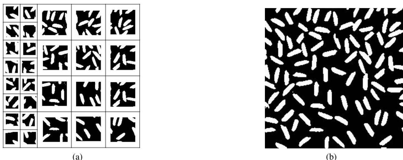
Figure 6: (a) Segmentation of subimages (b) Final Segmentation results of Rice image
