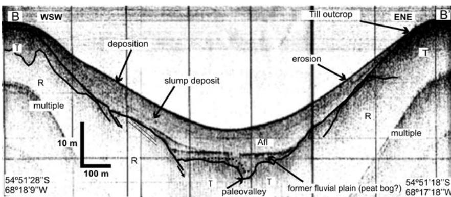
FIGURE 19 | WE subbottom seismic section along Golondrina Bay (Beagle Channel) performed with a 3.5 kHz profiler. R: Mesozoic metamorphic rocks; T: till (Bujalesky et al., 2004). See location in Figure 16.
