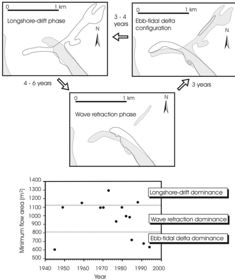
FIGURE 10 | Evolutionary cycle of Punta Popper spit and minimum flow areas of Rio Grande tidal inlet (areas below the mean tide level obtained after soundings performed by the Servicio de Hidrografía Naval, 1994). See location in Figure 7.
