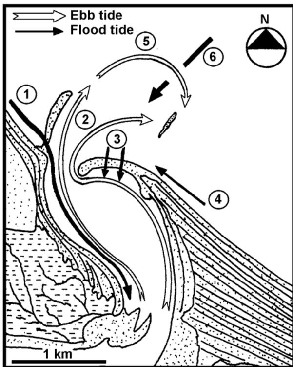
FIGURE 9 | Directions of sediment transport. 1) regional Atlantic littoral drift, during high tide; 2) sediment transport due to ebb tidal currents; 3) overwashing due to Atlantic swells at spring tide; 4) local littoral drift due to wave refraction; 5) interaction between ebb tidal currents with Atlantic waves; 6) landward migration of subtidal bars (Bujalesky, 1997b). See location in Figures 3 and 7.
