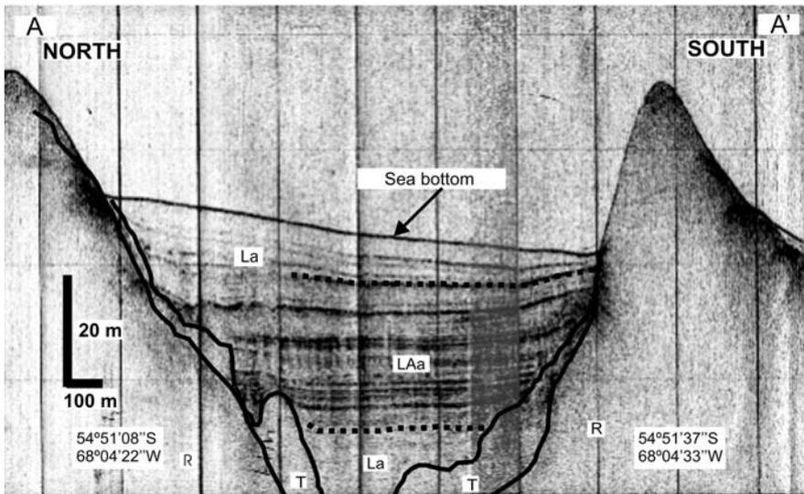
FIGURE 18 | N-S subbottom seismic section of the Beagle Channel from Punta Segunda to Les Eclaireurs Islands performed with a 3.5 kHz profiler. R: Mesozoic metamorphic rocks; T: till; A: gravelly sands; LAa: silty sands; La: sandy silts (Bujalesky et al., 2004). See location in Figure 16.
