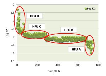
**FIGURE 8.** Log Flow Zone Indicator (FZI) versus sample numbers for determination of hydraulic flow units in the reservoir.
