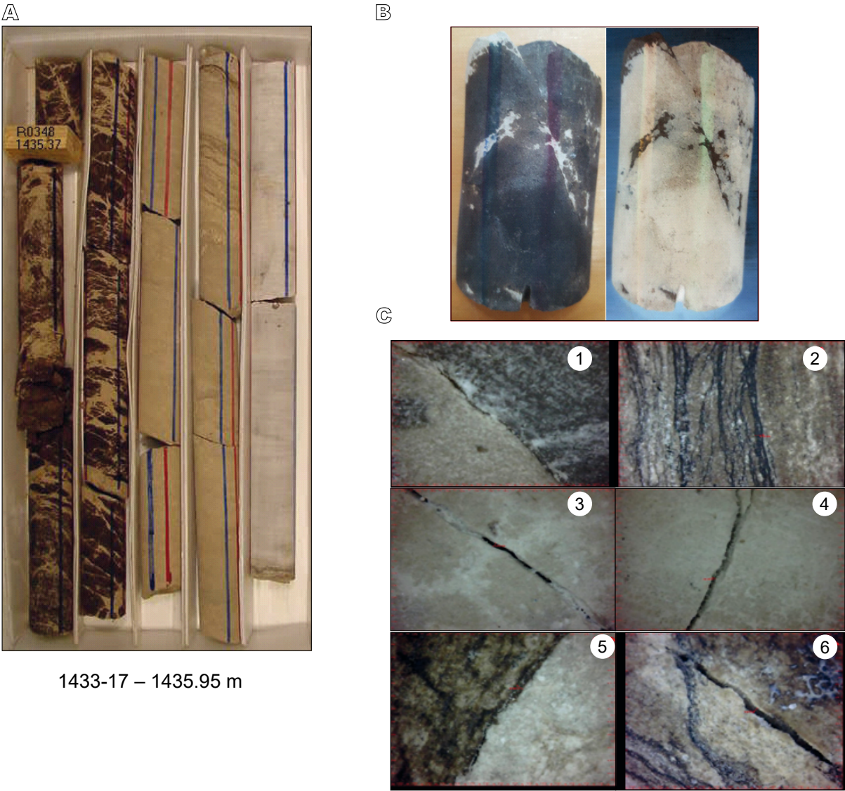
FIGURE 15. Fractures in the target carbonates show a wide range of lengths and thickness, with calcite infillings. A) representative microscope images of fractures. B) core box image of the oil-impregnated interval. C) fracture in the oil-impregnated interval.
