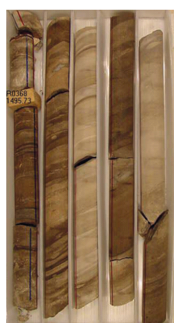
FIGURE 9. The pre-impact target carbonate sequence. Core box images and 3-D core scans of the impact breccia section.
