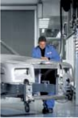
Inspecting the surface quality of an aluminium space frame body.
