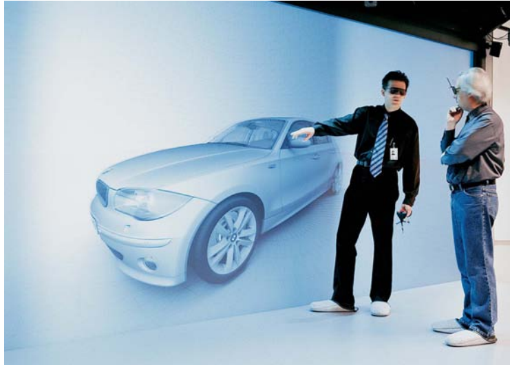
Virtual reality on the "Powerwall". Entire vehicles or individual parts can be displayed, examined and optimised in 3D, long before the first prototype is built.
