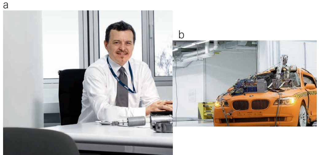
Image — a — Klaus Kompaß — Head of vehicle safety at the BMW Group. — b — After the crash — The new BMW 7 Series after a side impact at more than 56 km/h.
