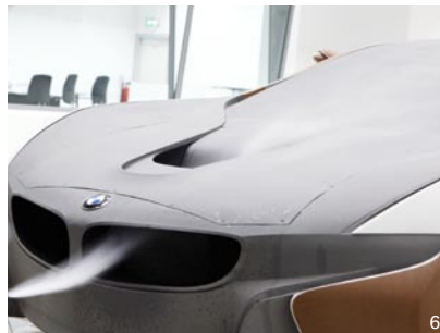
6 Flow optimisation for the Vision EfficientDynamics
