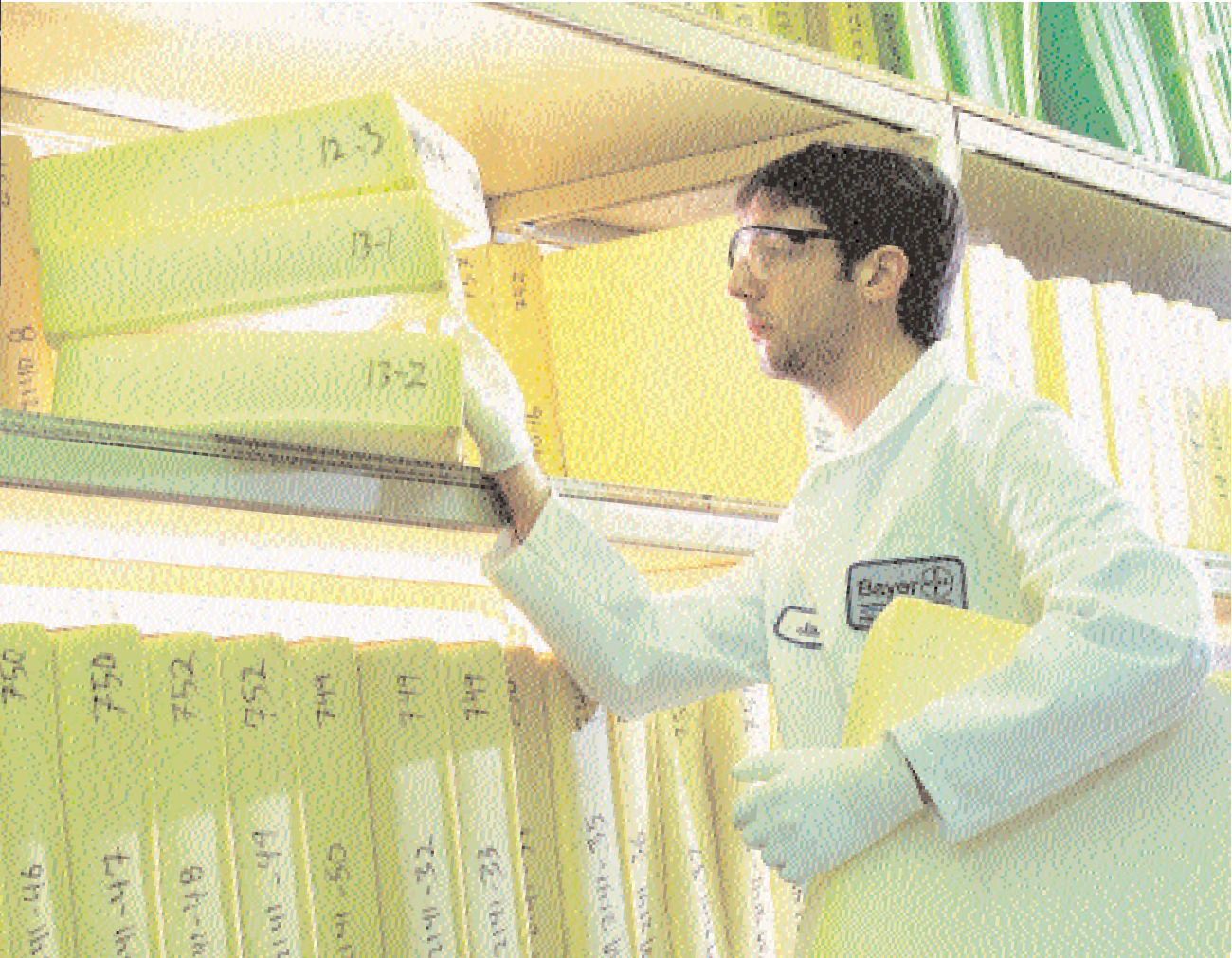
Slabs of different foams – carefully labeled and indexed – are left to dry for 24 hours before undergoing a series of tests to determine whether the materials meet customer specifications.
