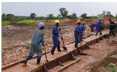
Miners using a sluicing technique to concentrate tantalite ore at the Mai Baridi Mine in Katanga Province, Democratic Republic of the Congo
