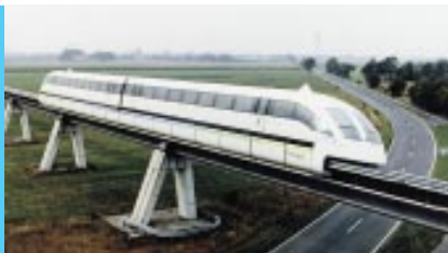
The German magnetic-levitation train system Transrapid – a vehicle on the test track in Emsland
