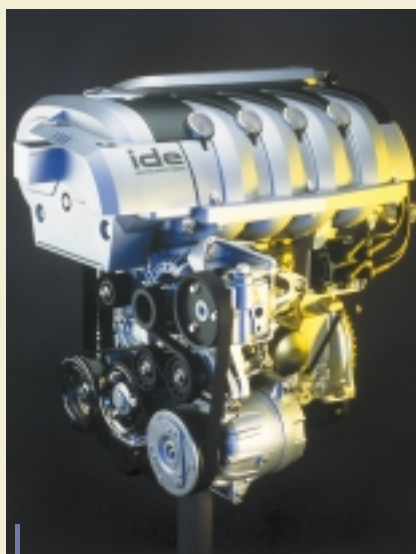
Derived from the 2.0 16V "F4R", the standard unit of the Espace, Laguna and Scenic, the 16-valve F5R with twin camshaft and direct gasoline injection (IDE), was a joint development with Renault Sport. The result, for the Mégane Coupé and Cabriolet, is a versatile and lively engine which gains in driving pleasure and fuel economy without the slightest compromise in terms of emission control.
