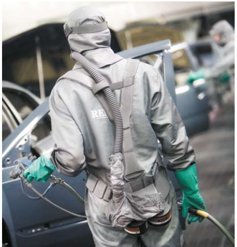
The paint used at Renault's Sandouville plant is water soluble, helping to limit the environmental impact.
