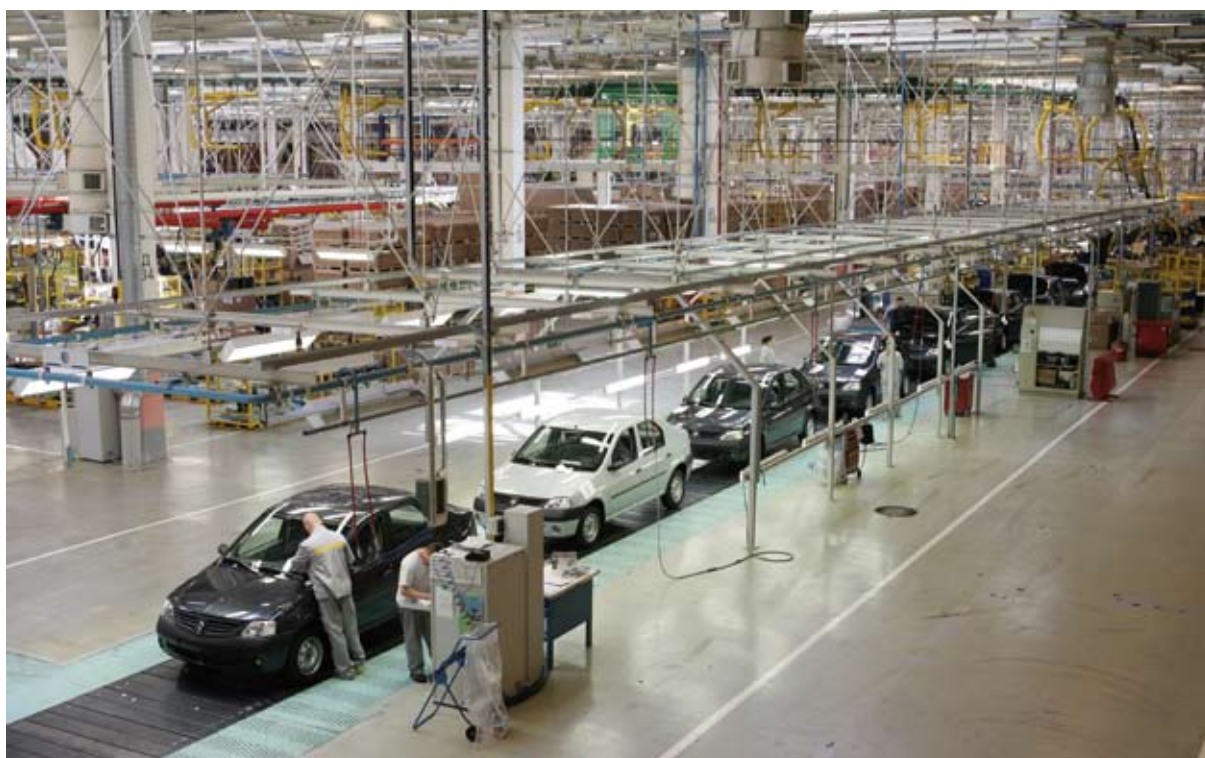
Tune-up at the end of the Renault Logan assembly line at the Avtoframos factory in Russia.
