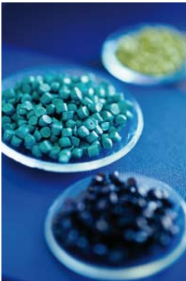
The search for recyclable materials is an integral part of Renault's quality approach. Recycled plastics are delivered in pellet form, as shown here.
