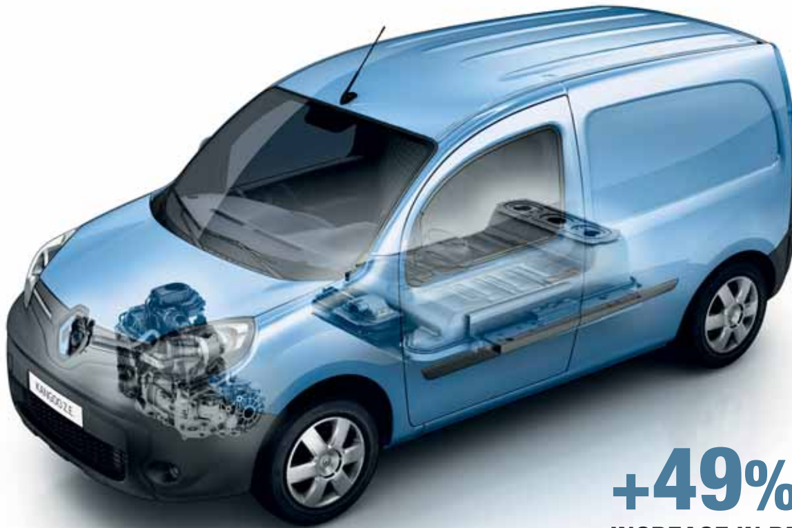
▲ Layout of the motor and battery on Kangoo Express Z.E.
