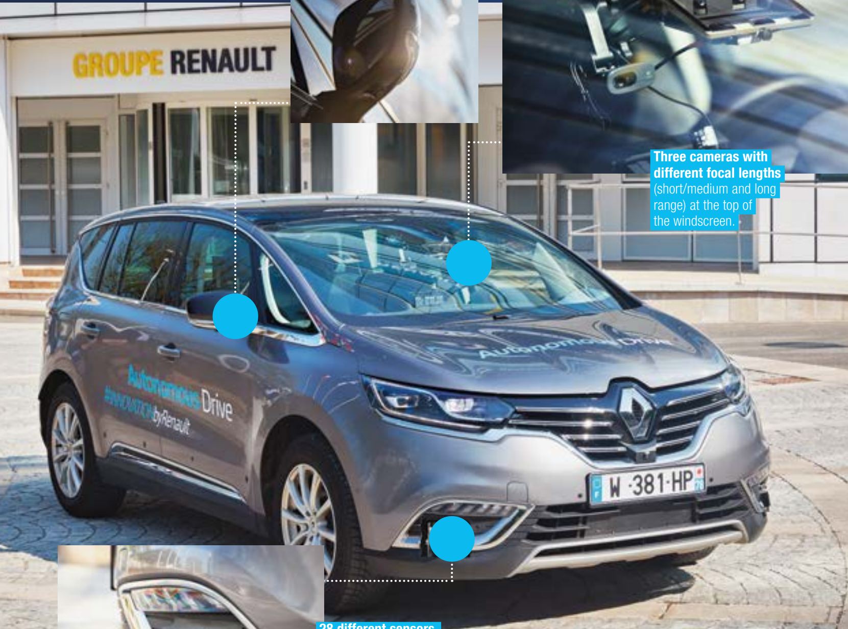
28 different sensors, corner radars, a long-range central radar and LIDARs are part of the range of sensors found on the autonomous Espace.
