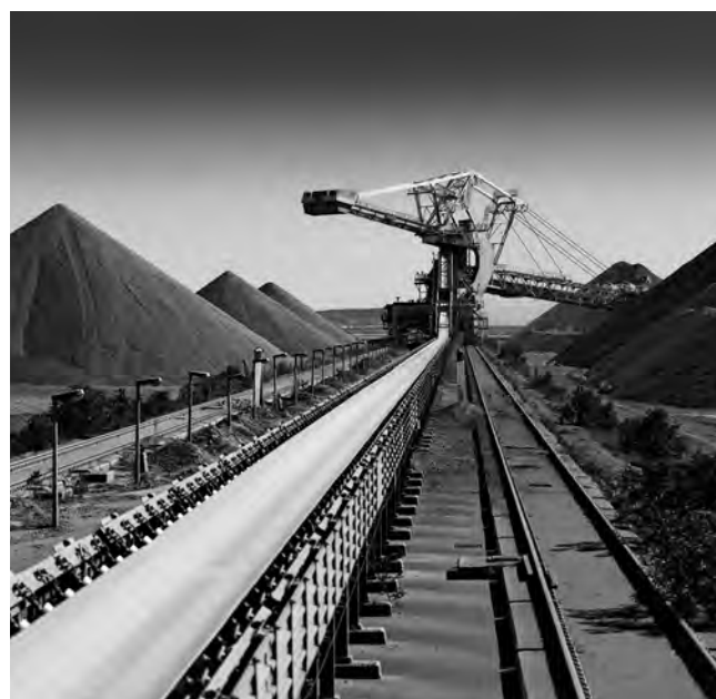
At Sishen, ore stockpiles are controlled by four stacker/reclaimers. Mining operations have been substantially reconfigured to reduce waste and to make the overall operation more resilient to future deteriorations in the iron ore price.
