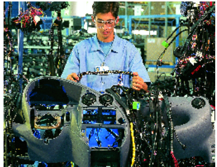
Samuel William de Sales installs an AFL wire harness.
