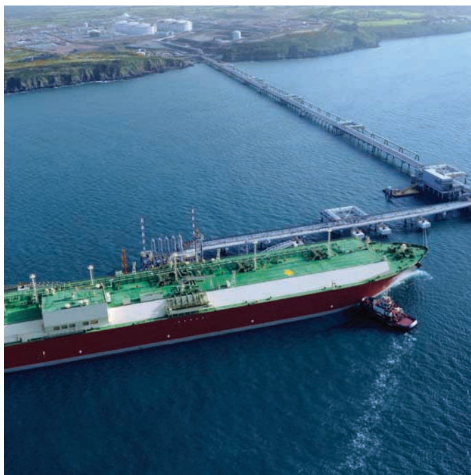
The Q-Max carriers are longer than three football fields, tower 20 stories tall from keel to masthead, and are equipped with the largest membrane containment tanks ever built. With a total capacity of up to 266,000 cubic meters, each ship carries enough natural gas to meet the energy needs of 70,000 U.S. homes for one year.
