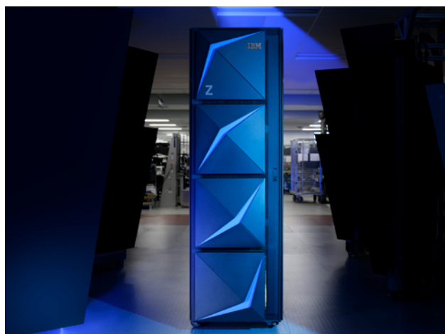
IBM's new z15 mainframe system uses 20-30% less power than its predecessor, the z14.
