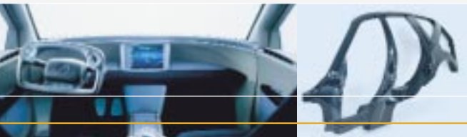
Z22 lightweight cockpit and side frames made from carbon fiber reinforced polymer (CFRP)
