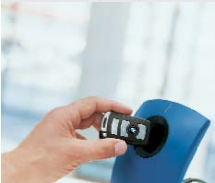
[above] Mobile diagnostics equipment in use [below] Vehicle data can be transmitted electronically with the ignition key.
