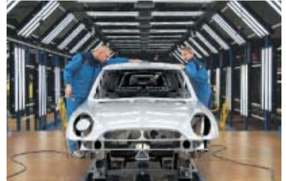
MINI production in Oxford: paint quality control
