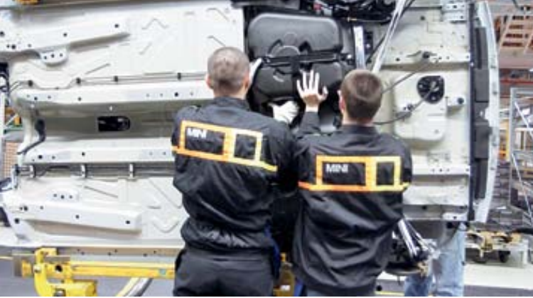
above -- Swivelling assembly enables employees to fit the tank while standing and thus reduces physical strain. below -- Height-adjustable workbenches in cable harness assembly relieve the strain on back and knees.
