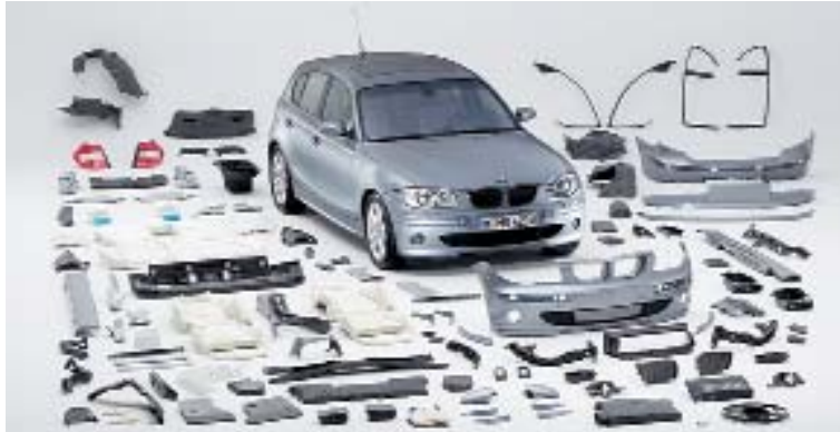
above -- Recycling-optimised plastic components of the BMW 1 Series below -- Fitting a luggage compartment panel made of renewable raw materials
