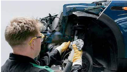
Oil removal from shock absorbers: The recycling experts of the BMW Group have developed in partnership a device for the rapid and safe evacuation of the old oil.
