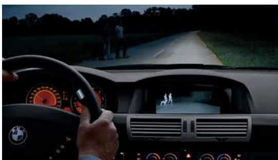
More safety in the dark. With BMW Night Vision, obstacles outside the light cone of the headlights can be detected early.
