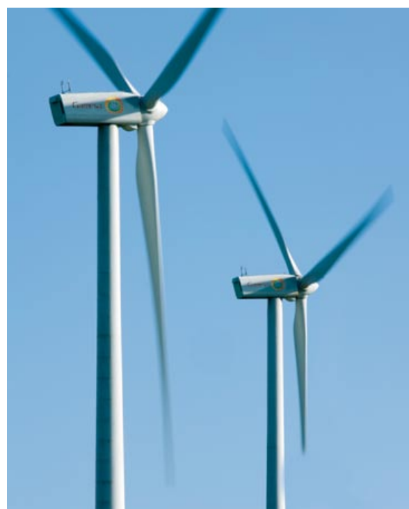
Aerogeneradores Gamesa G90-2.0 MW.
