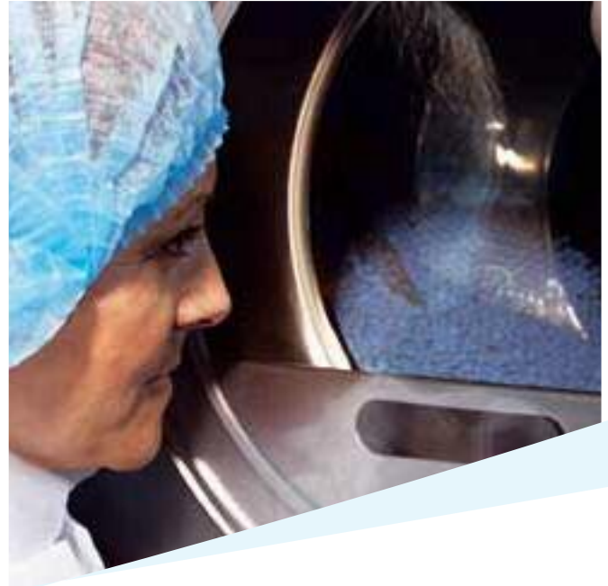
Coating tablets in a film-coating machine
