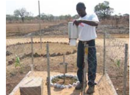
Under the flood-warning system, precipitation levels are measured daily and critical readings reported.
