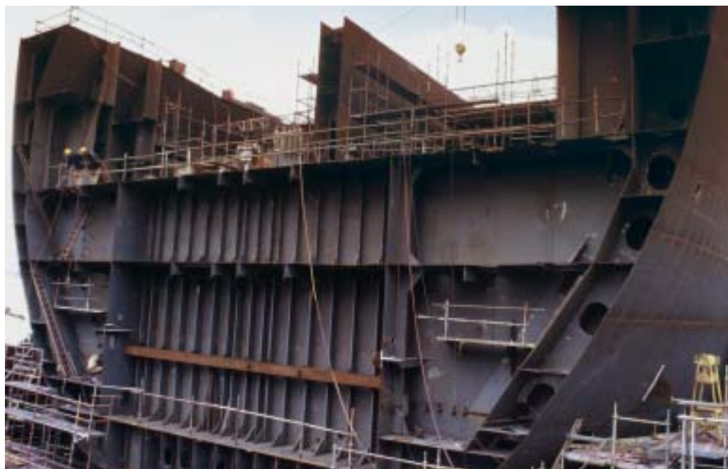
Cross-section of a double hull. The narrow and winding space between the two steel hulls must be properly protected with a coating of special paint to prevent the steel from rusting.
