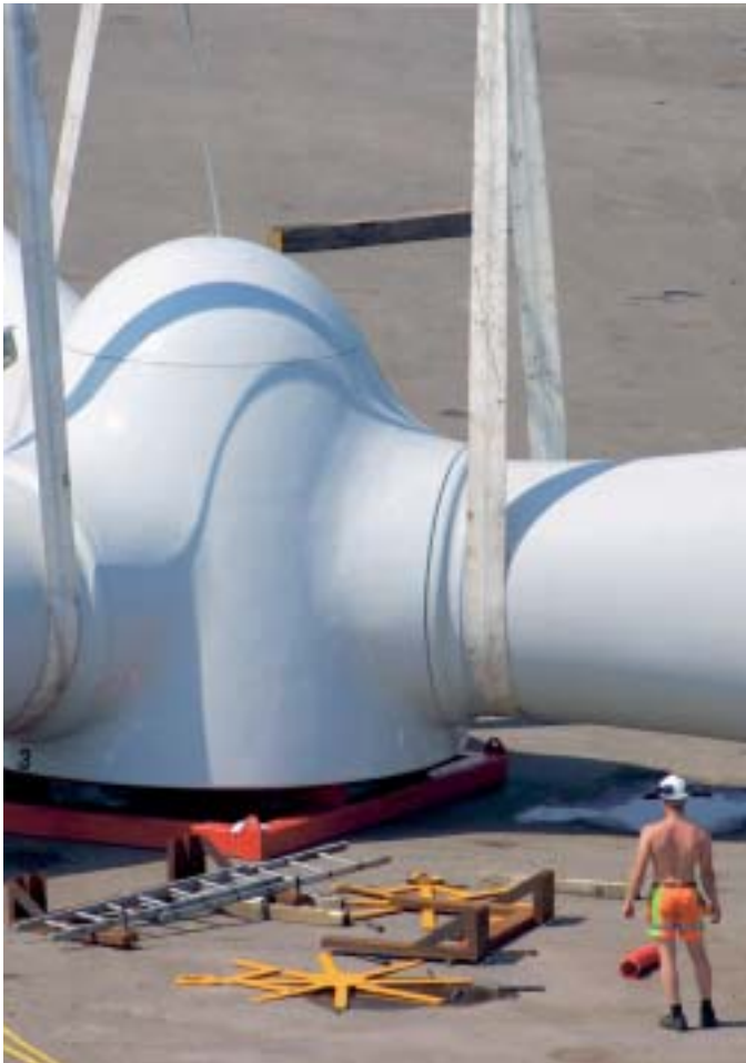
Rotor hub of a turbine at Horns Rev wind farm. One blade weighs 6.5 t.
