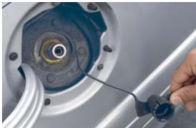
Filling up with natural gas is easy – and when the tank is empty, the engine automatically switches over to using petrol.
