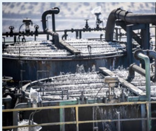
The coarse particle flotation process is already being used at Las Tórtolas, part of the Los Bronces copper mine, in Chile.
