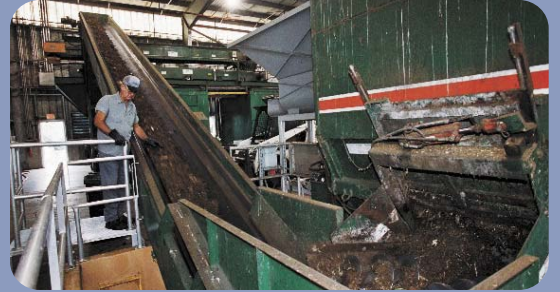
Food waste is mixed with wood chips in a hopper and then transported to reactor tunnels in an in-vessel compost system where they break down naturally. Cast Members monitor the system to remove noncompostable materials.
