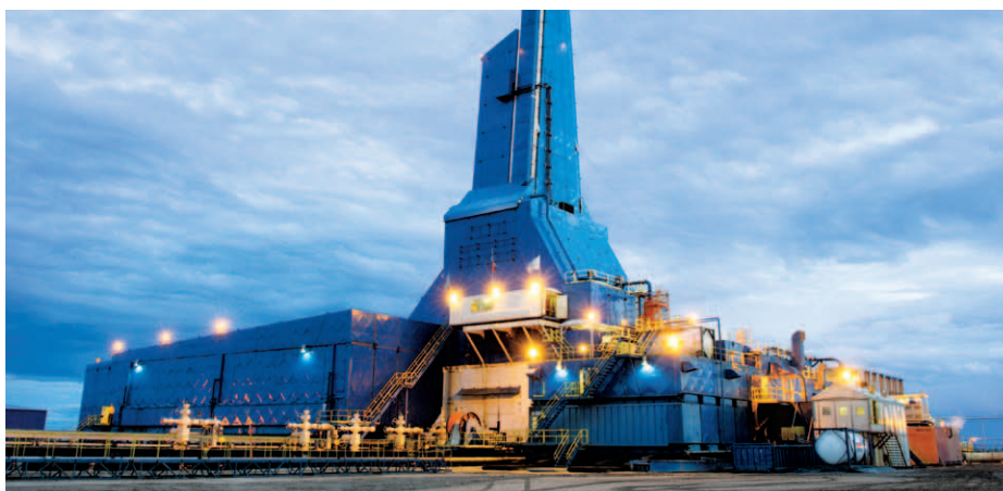
In Sakhalin, Russia, leading-edge technology was applied to drill extended-reach wells from the shoreline to the Chayvo field. This allowed for horizontal drilling under the sea floor and eliminated the need for a second offshore platform while minimizing and in some cases eliminating environmental risks.
