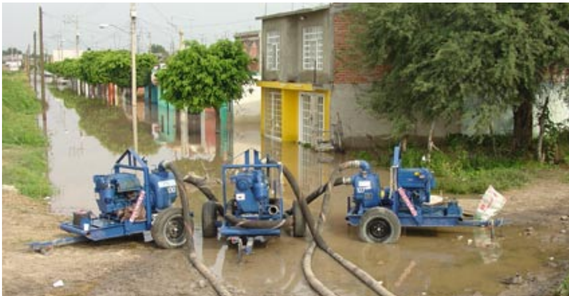
Donated machinery is used to pump out floodwaters from residential areas in the Guanajuato region of Mexico.
