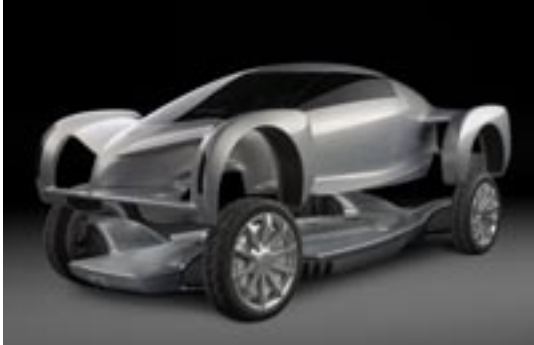
The AUTonomy skateboard design demonstrates the many possibilities available when building a car with fuel cell and by-wire technology.
