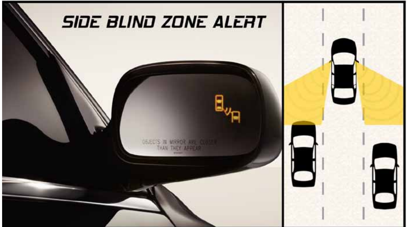
Side blind zone alert uses radar sensors to warn drivers of an object in their blind spot.
