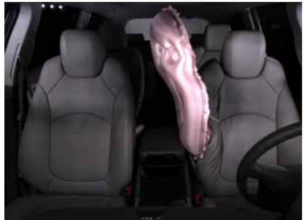
The industry's first front center air bag will help protect drivers and front passengers in far-side impact crashes where the affected occupant is on the opposite, non-struck side of the vehicle.
