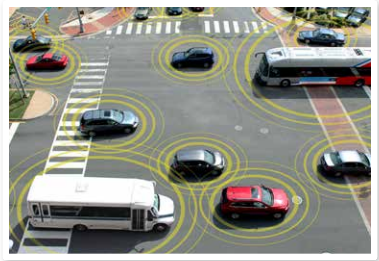
Vehicle-to-vehicle communications technology allows cars to send and receive information such as location, speed and direction of travel, and could help mitigate future collisions and congestion.
