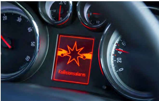
A camera-based front alarm combines audible warnings with a visual display on the dashboard to warn a driver who is following too closely or about to change lanes without signaling.
