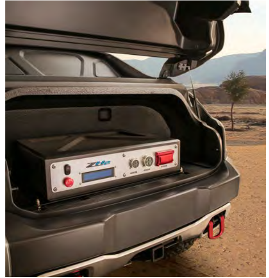
Inside the rear hatch of the Chevrolet Colorado ZH2 fuel cell electric vehicle is an Exportable Power Take-Off unit, capable of providing 25 kW of consistent electric power away from the vehicle in remote locations where electric power may otherwise be unavailable.
