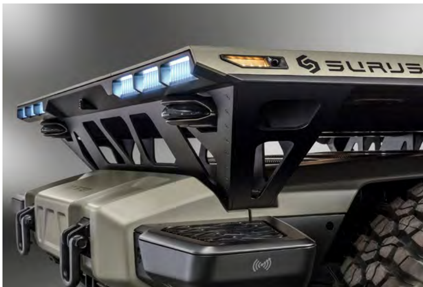
The Silent Utility Rover Universal Superstructure (SURUS) platform is a flexible fuel cell electric platform with autonomous capabilities. SURUS was designed to form a foundation for a family of commercial vehicle solutions that leverages a single propulsion system integrated into a common chassis.
