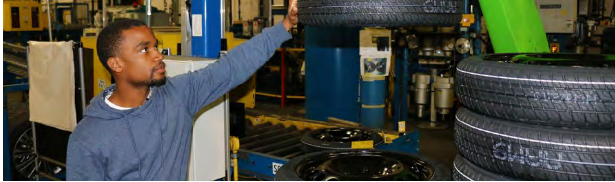
UAW Local 5960 member Byron Garrett demonstrates the safety of General Motors' first fully collaborative robot that is touch-safe for employees to work alongside without a safety cage. Replacing an ergonomically unfriendly job, the robot separates and stacks spare tires for Chevrolet Sonics and Buick Veranos. Plant management, union officials and safety representatives worked closely together to comply with all safety requirements and implement this cutting-edge technology.
