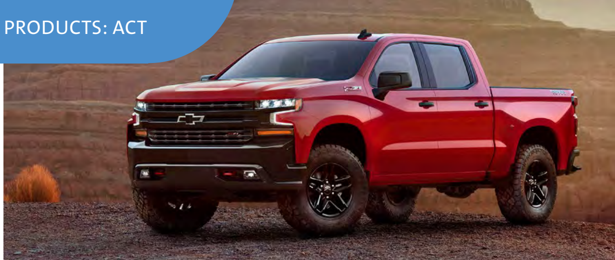
The 2019 Chevrolet Silverado is up to 450 pounds lighter than the previous model through use of mixed materials.
