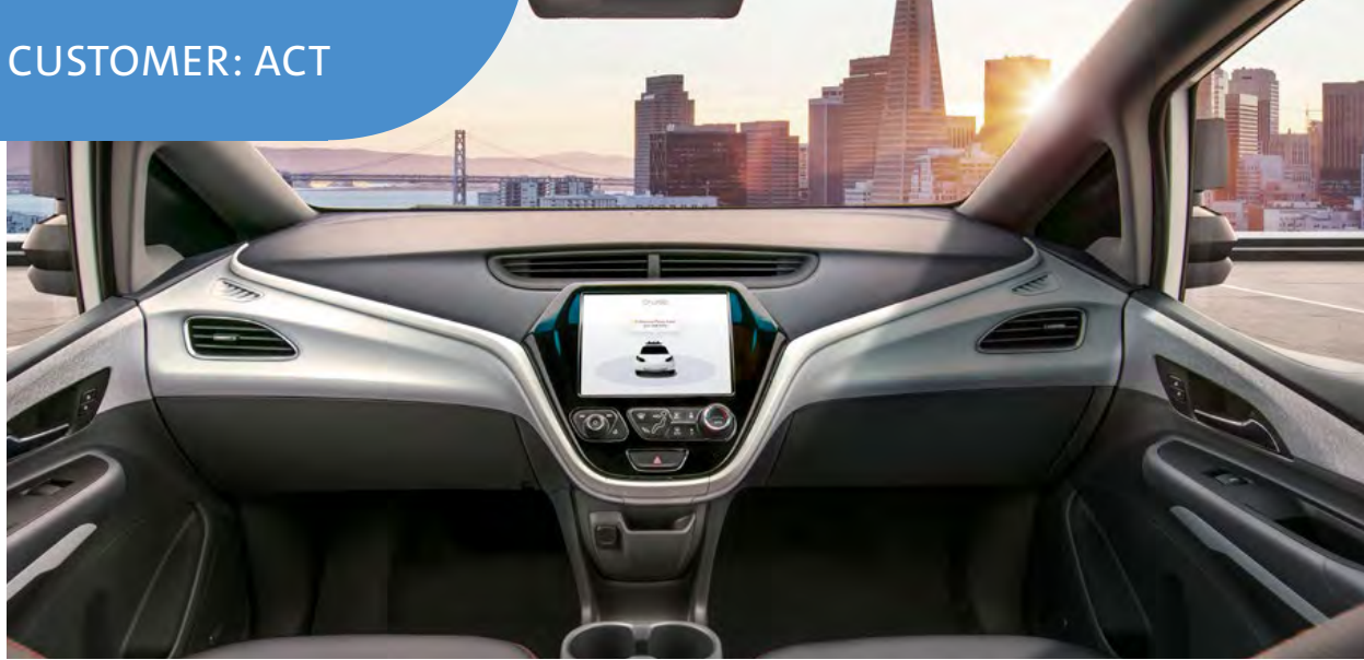
The Cruise AV is designed to operate on its own, with no driver, steering wheel, pedals or other manual controls.
